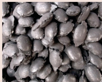
Briquettes from sponge iron fines with a density of 5 grams/cc
