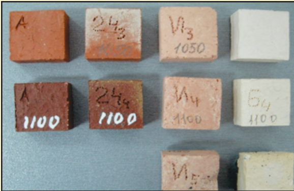
Bricks made in the laboratory, using different clay types & different firing temperatures
